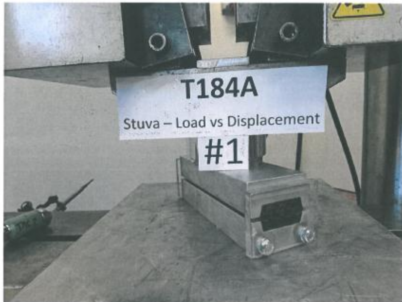
Photo 1: T184A Under Test at offset 0mm
