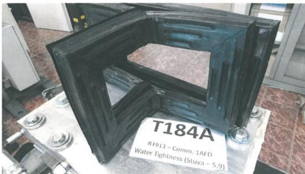
Photo 3: Sample after test and corner detail
