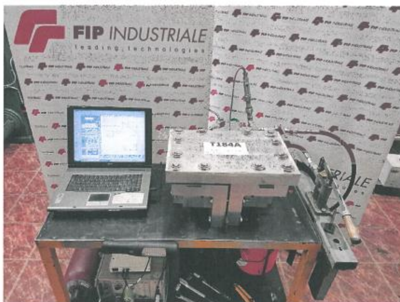
Photo 2: Assembled Test Rig + Pressure control system + DAQ
