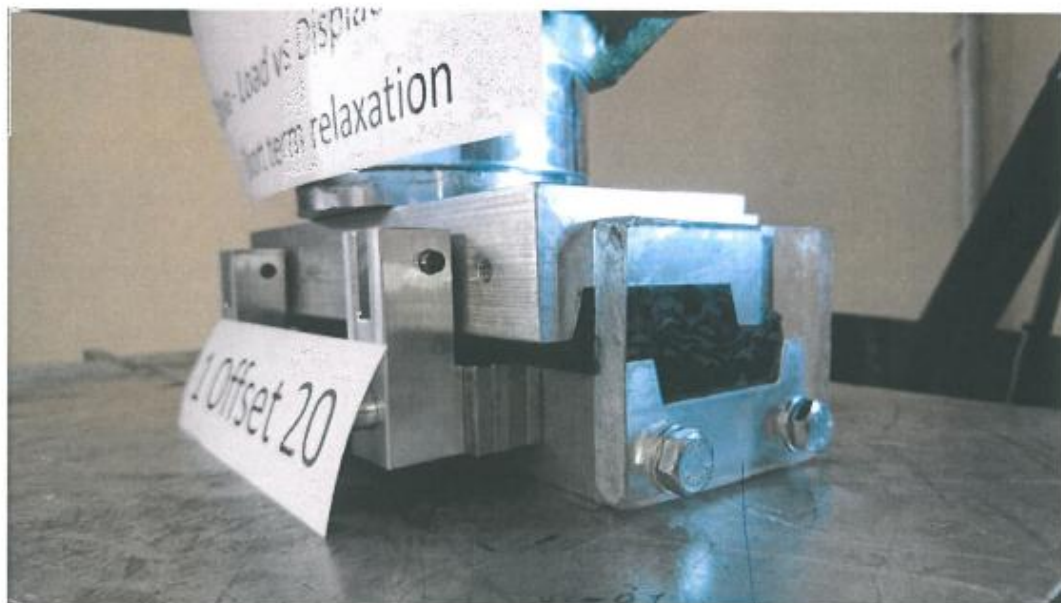
Photo 2: T184A Under Test at offset 20mm
